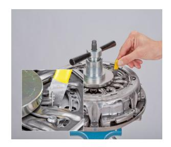
• Release and unscrew the pressure nut
