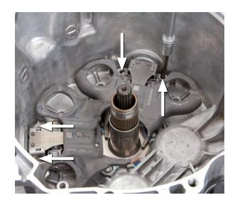
• Remove both lever actuators
